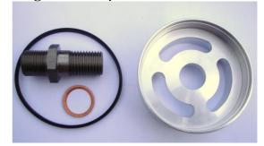
Remove the bolt, bowl, and old oil filter. Remove the large seal which sits in the groove in the filter head - it may be a tight fit. Ensure the groove is clean and no debris remains. Remove the steel centre boss by placing a tommy-bar through the holes in the side and unscrewing it. Remove the splash plate (if fitted).
